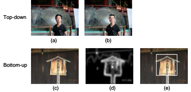
Figure 5. The process of ROI determination. (a)(c) The original photo, (b) face detection result, (d) saliency map derived from color contrast, (e) attentive region derived from the saliency map.
